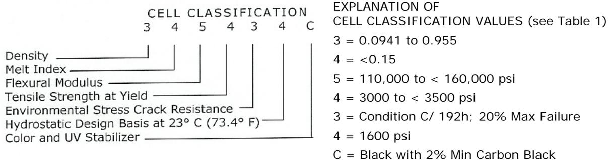
Table 1 of ASTM D 3350 lists the primary properties of the Cell Classification and paragraph 6.2 of D 3350 indicates the color and UV stabilizer codes.
