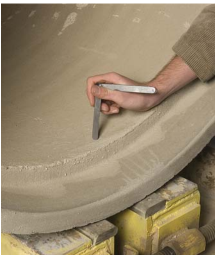
The 0.04-inch crack shown is less than half the crack width of 0.10-inch accepted by Caltrans and AASHTO.
