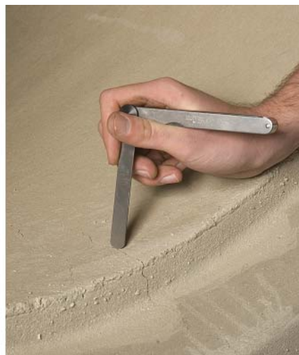
The 0.04-inch crack shown is less than half the crack width of 0.10-inch accepted by Caltrans and AASHTO.
